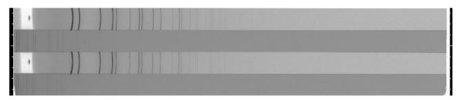
(d) 2-dimensional diffraction data of aluminum at 500 and 600 K.
