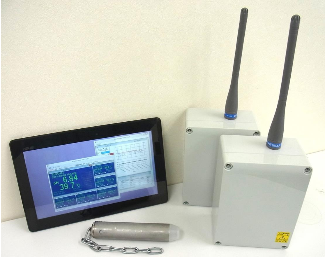
Fig. 4.2 Wireless radio transmission pH measurement system (DKK-TOA Yamagata Corporation, Yamagata, Japan)
