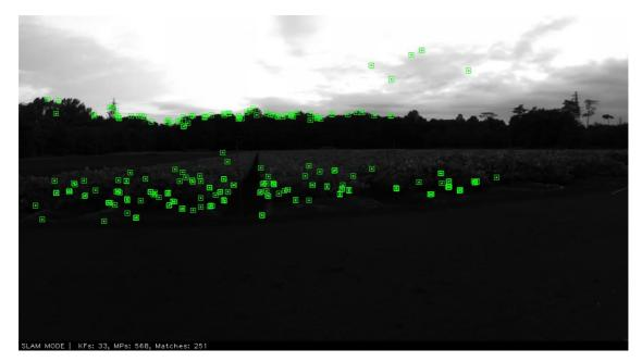
Figure 5.13. ORB features detected by ORB-SLAM system using ZED camera to navigate the EPV
