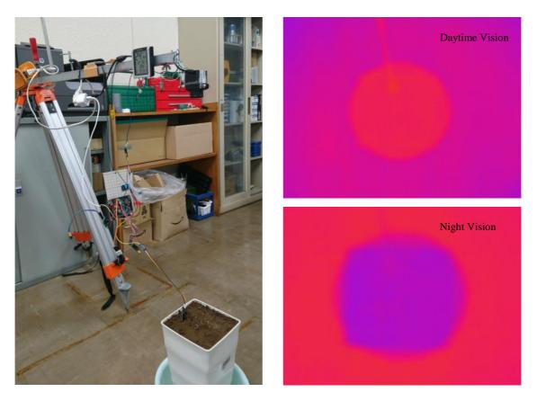
Figure 4.9. Soil Moisture Change Monitoring System and Thermal Images
