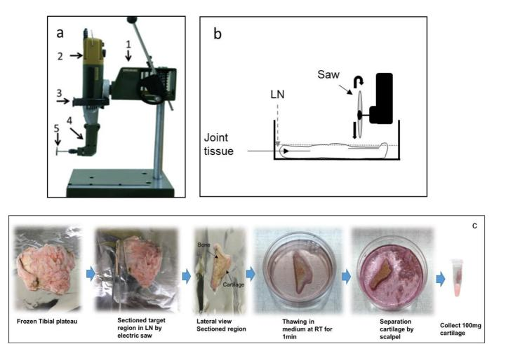
Figure 2-4 Custom tools for frozen joint tissue sectioning and cartilage separation.
