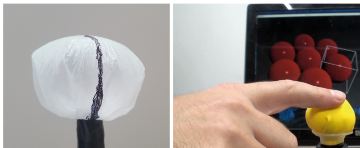
Fig. 6.19. The implementation of the capacitive touch sensor. On the left, the internal air-bag; on the right, a test with a 3d simulation.
