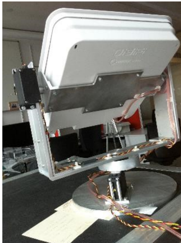
Figure 2.6: The custom built pan tilt gimbal holding the parametric speaker.
