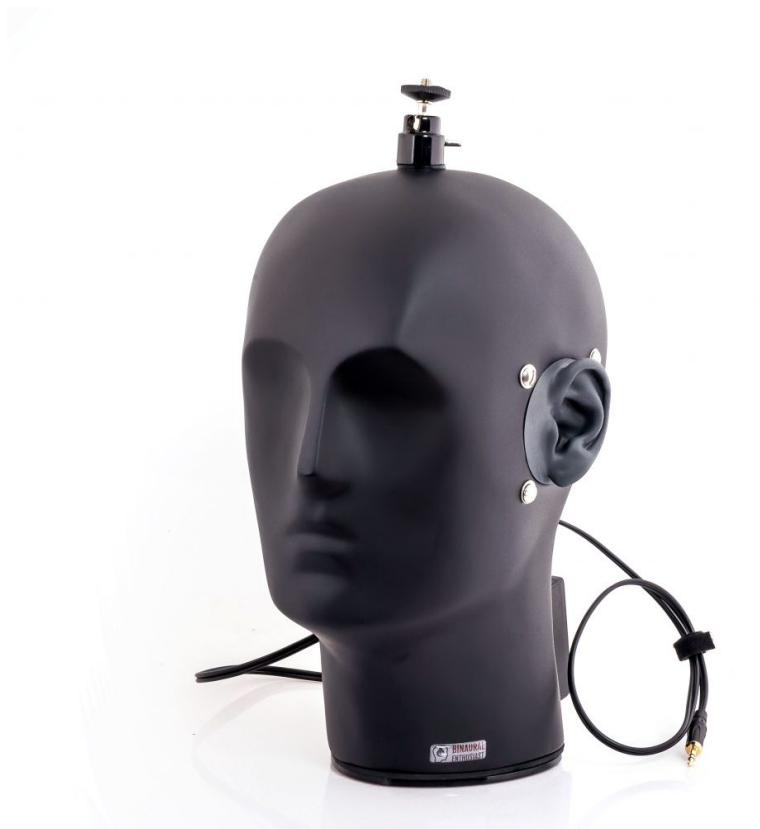
Figure 2.2: An example of a binaural recording unit. Microphones are embedded in the cavity of the ears.
