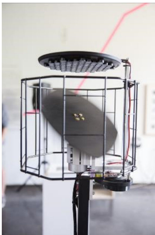
Figure 2.8: The spinning reflector allows audio to be positioned horizontally about the unit.
