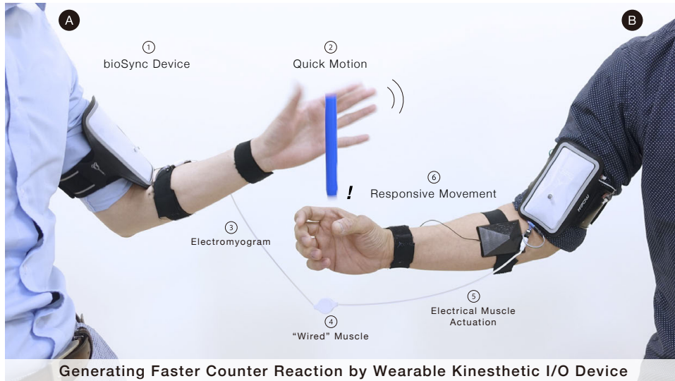
FIGURE 6.23: Wired Muscle: a system for directly connecting muscles of two persons. The EMG detects the muscle activity of a person A, which triggers the EMS to drive the muscle of person B to produce rapid corresponding movements.
