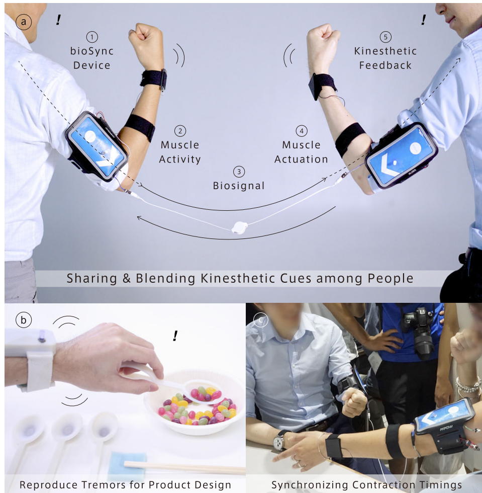
FIGURE 3.4: (a) Synchronizing and combining muscle activities among people (b) Reproducing kinesthetic experience of Parkinson's impairment for use in supporting product design (c) Participants express surprise when the muscle activity is jacked in by the demonstrator
