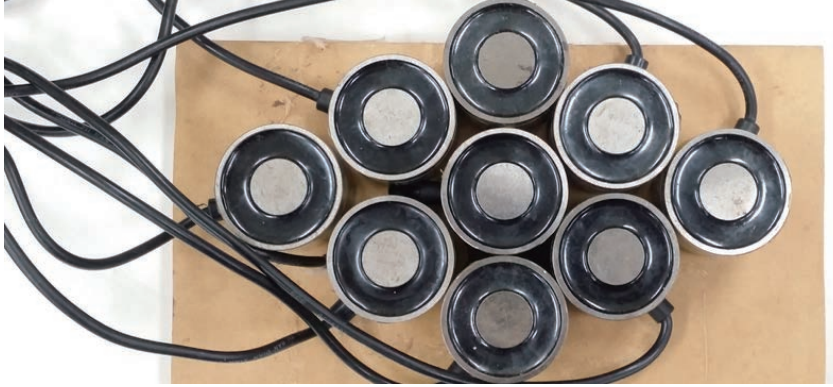
FIGURE 3.4: Arrangement of electromagnets used for transporting solid objects.
