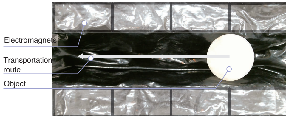
FIGURE 5.13: Channel transportation route. The robotic sheet is set on channel-like surface. By activating the electromagnets and changing the inner surface of the channel, the ball is moved from right to left. [ Tone et al., [92], p.9 ]
