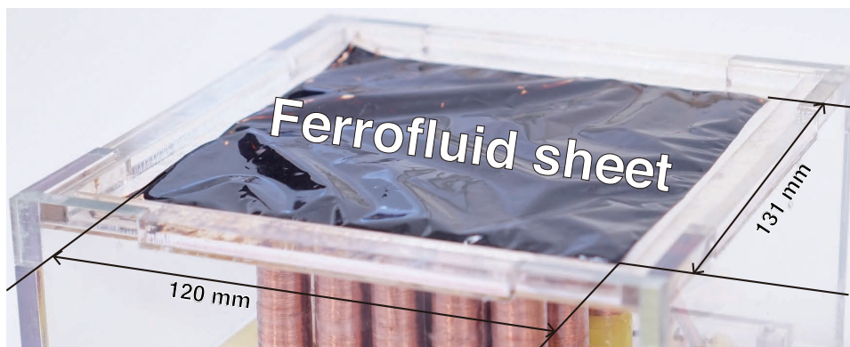
FIGURE 3.2: The ferrofluid-based deformable robotic sheet for flexible objects. Polytetrafluoroethylene films are used as the thin film and a ferrofluid is wrapped with the films. [ Tone et al., [91], p.2816 ]
