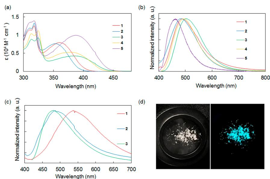
**Figure 2.** (a) UV-vis absorption spectra of **1–5** in  $\text{CH}_2\text{Cl}_2$ . (b) Photoluminescence spectra of **1–5** in  $\text{CH}_2\text{Cl}_2$ . (c) Photoluminescence spectra of **1–3** in the solid state. (d) Photographs of **2** in the solid state. Left: under ambient light. Right: under UV light ( $\lambda_{\text{ex}} = 365 \text{ nm}$ ).
