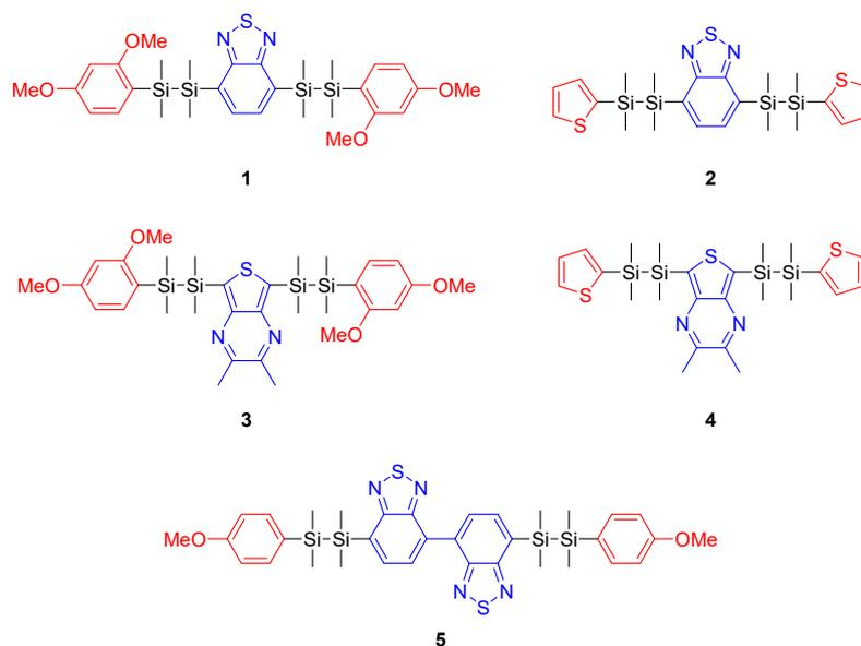
**Figure 1.** Chemical structures of disilane-bridged D/A/D molecules synthesized in this work. Red marked groups: aromatic electron-donating substituents. Blue marked groups: aromatic electron-accepting substituents.
