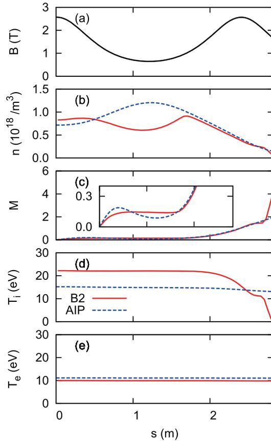
Fig. 4 Profiles of plasma parameters for the lowest collisionality case in Fig. 2 (i.e.  $L/\lambda_{\text{mp}} \approx 0.3$ ) of the B2 code (solid lines) and the AIP model (broken lines); (a)  $B$ , (b)  $n$ , (c)  $M$  with an enlarged view, (d)  $T_i$  and (e)  $T_e$ .
