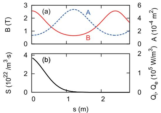
Fig. 1 Calculation conditions used in this paper; parallel-to- $B$  profiles of (a)  $B$  (solid line),  $A$  (broken line) and (b) source terms in the case of  $S_0 = 3.70 \times 10^{22} / \text{m}^3 \cdot \text{s}$  and  $T_{\text{in}} = 20$  eV.
