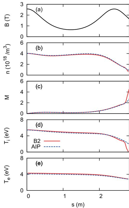
Fig. 3 Profiles of plasma parameters for the highest collisionality case in Fig. 2 (i.e.  $L / \lambda_{\text{mfip}} \approx 30$ ) of the B2 code (solid lines) and the AIP model (broken lines); (a)  $B$ , (b)  $n$ , (c)  $M$ , (d)  $T_i$  and (e)  $T_e$ .
