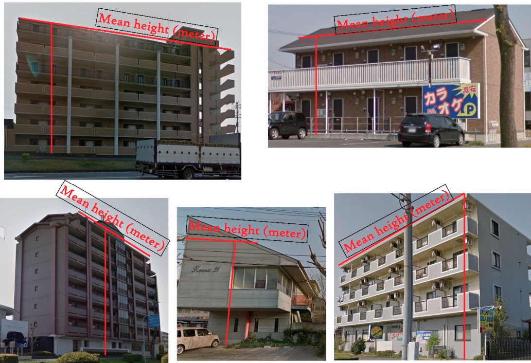
Fig. 6. Measuring building heights by using SFH (Source: Google Street map, 2018).
