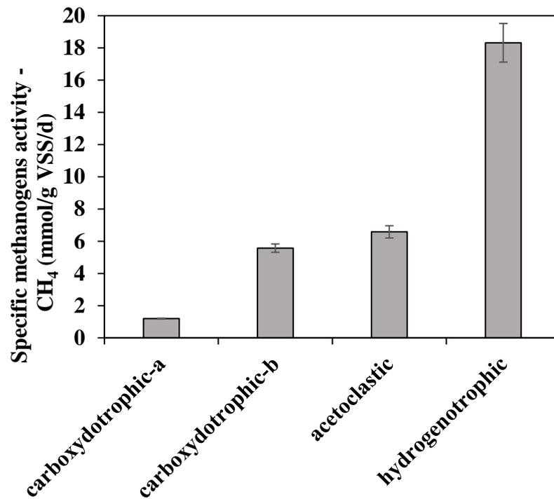
Fig. 3-2 Anaerobic biomethanation potential of AGS used in this study at 37°C. The substrates for carboxydrotrophic-a, carboxydrotrophic-b, acetoclastic, and hydrogenotrophic activities were CO/N<sub>2</sub>, CO/CO<sub>2</sub>/H<sub>2</sub>, sodium acetate, and H<sub>2</sub>/CO<sub>2</sub>, respectively.
