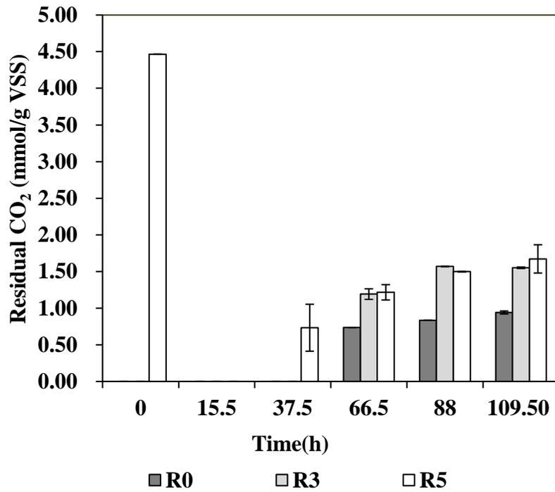
Fig. 3-5 Anaerobic biomethanation potential of AGS at 37°C: CO<sub>2</sub> consumption and production. (R0-control, R3-CO/N<sub>2</sub>, R5-CO/CO<sub>2</sub>/H<sub>2</sub>)
