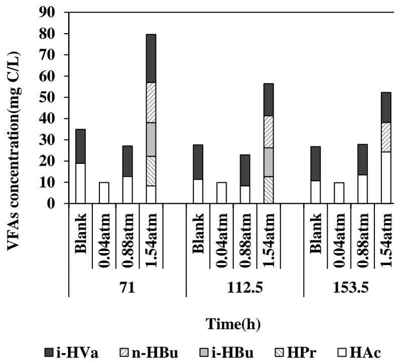
Fig. 3-14 Effect of H<sub>2</sub> partial pressures (atm) on VFAs distribution during BFG fermentation by AGS at 37°C.
