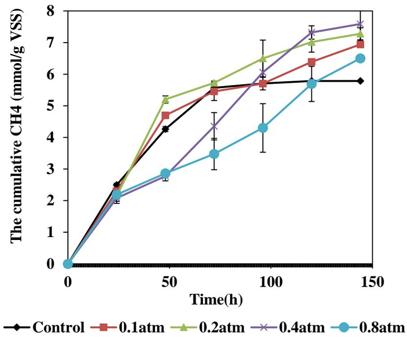
Fig. 3-7 Effect of CO partial pressures (atm) on methane production from CO by AGS.
