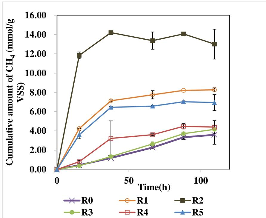
Fig. 3-3 Anaerobic biomethanation potential of AGS at 37°C: CH<sub>4</sub> production (R0-control, R1-sodium acetate, R2-H<sub>2</sub>/CO<sub>2</sub>, R3-CO/N<sub>2</sub>, R4-CO/H<sub>2</sub>; R5-CO/CO<sub>2</sub>/H<sub>2</sub>)
