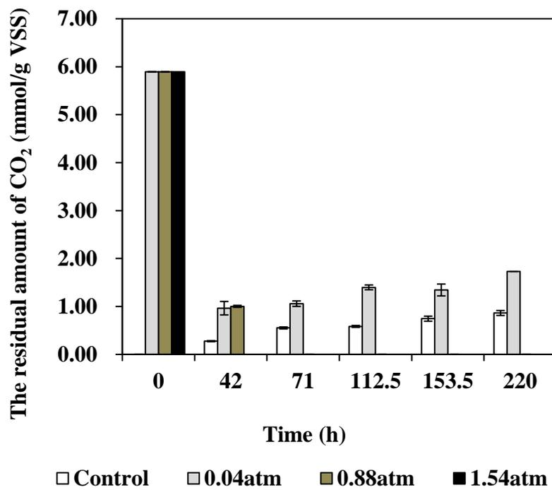
Fig. 3-13 Effects of H<sub>2</sub> partial pressures (atm) on residual CO<sub>2</sub> during BFG fermentation by AGS at 37 °C.
