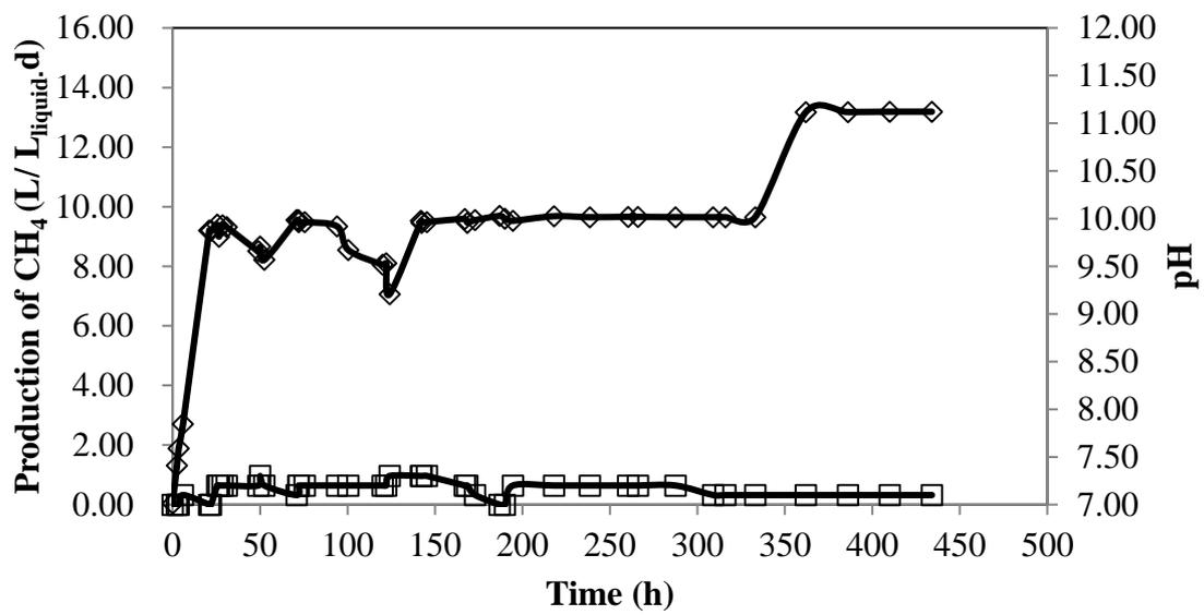
Fig. 2-6 CH<sub>4</sub> production rate (L/L<sub>liquid</sub> d) (◇) and pH (□) changes in the semi-continuous reactor.
