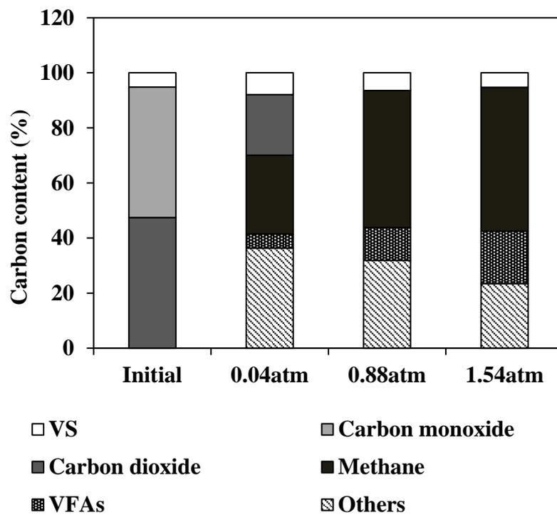
Fig. 3-15 Carbon balance analysis at different H<sub>2</sub> partial pressures during BFG fermentation by AGS on day 7.
