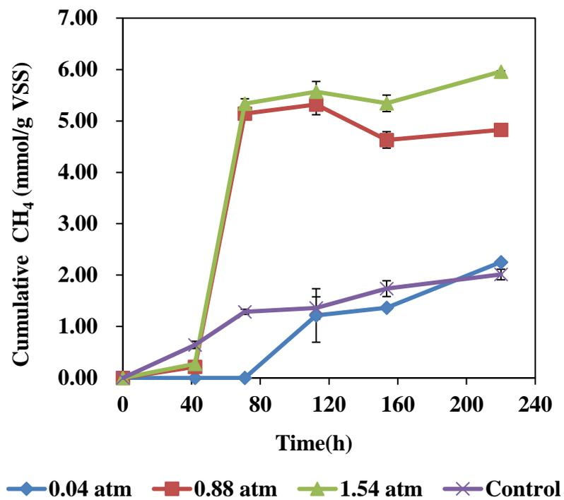
Fig. 3-12 Effects of H<sub>2</sub> partial pressures (atm) on cumulative CH<sub>4</sub> during BFG fermentation by AGS at 37 °C.
