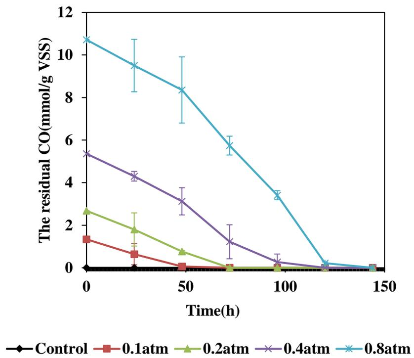
Fig. 3-8 Effect of CO partial pressures (atm) on CO consumption by AGS.
