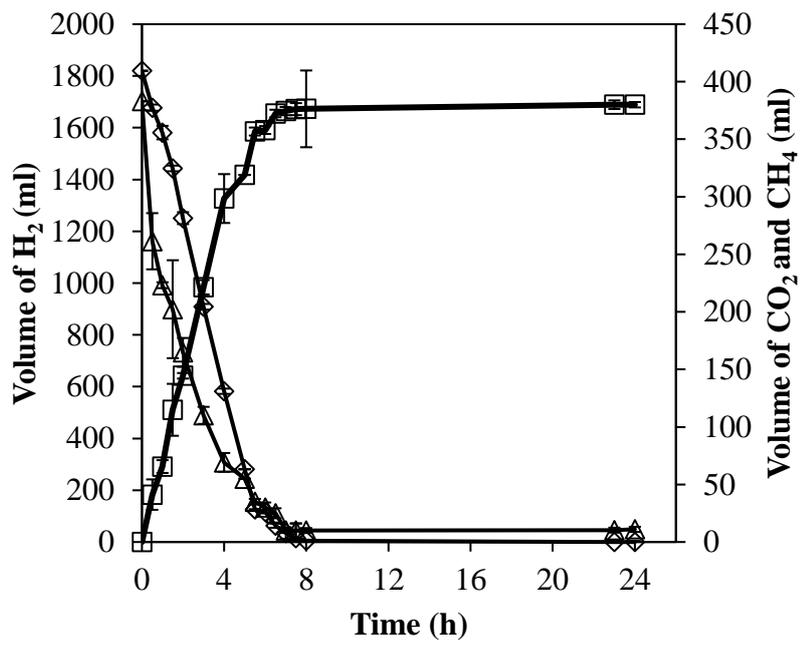
Fig. 2-3 H<sub>2</sub> and CO<sub>2</sub> consumption and CH<sub>4</sub> production profiles. H<sub>2</sub> (○), CH<sub>4</sub> (□), CO<sub>2</sub> (Δ).
