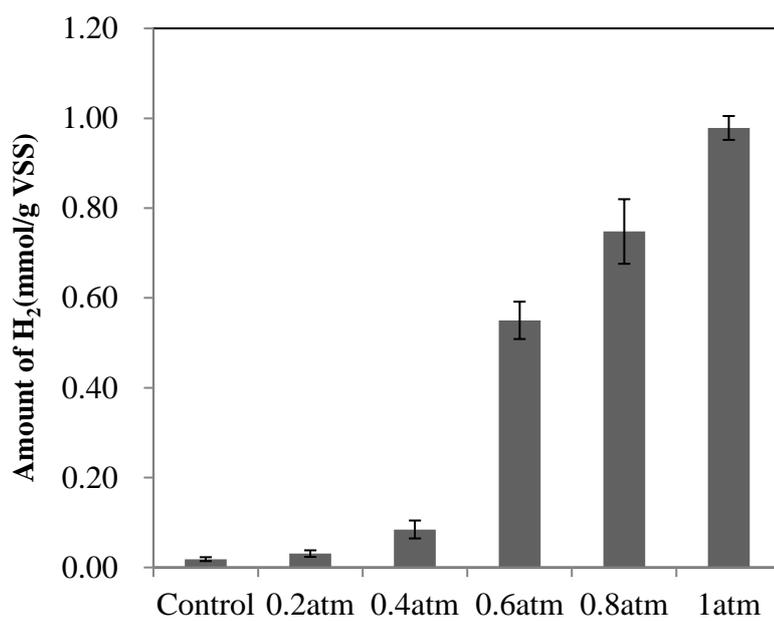
Fig. 3-11 Hydrogen accumulation under different CO partial pressures (atm) in the presence of BES at 37 °C.
