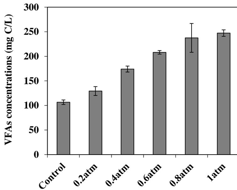
Fig. 3-9 Effect of CO partial pressure (atm) on intermediates formation from CO in the presence of BES at 37°C on day 7.
