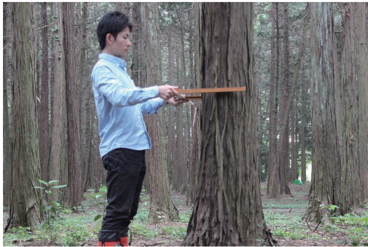
Fig. 5.8 Measuring diameter at breast height by the trunk caliper.
