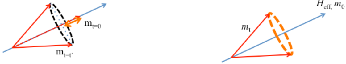
Figure 5.5.5 the schematic illustration for Photoresistance effect and rectification effect through AMR effects. The orange arrow and dashed circle induce the time-independent voltage.
