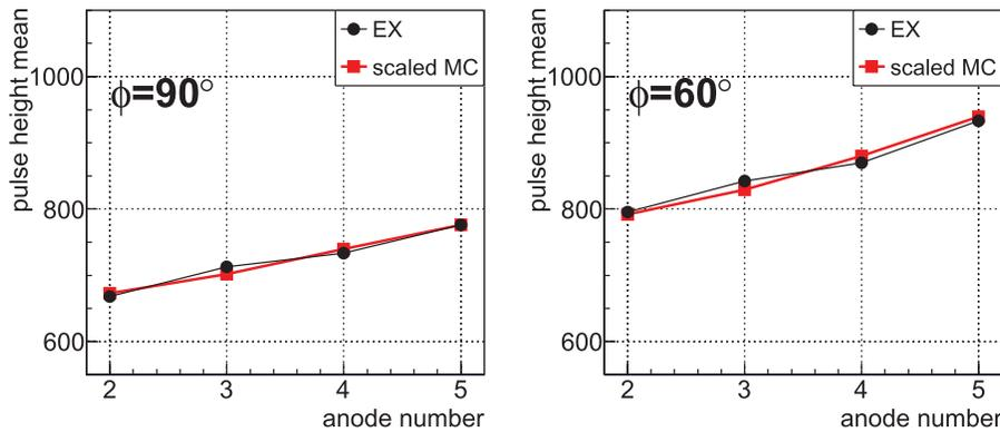
**Fig. 9.** Comparison of the anode pulse height from experiment (black) and the energy deposit calculated by the Monte Carlo simulation (red) for  $E_p = 2.00$  MeV.  $\phi$  was set between  $40^\circ$  to  $90^\circ$ , and  $V_0 = 1350$  V was applied. Here, the distribution of the calculated energy deposit was normalized so that its integral is in accordance with that of the experimental distribution.
