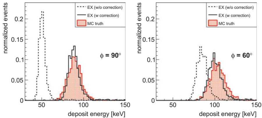
**Fig. 13.** Comparison of the energy deposit distribution without and including the correction for the gain reduction model. The distribution is obtained at anode wire 4,  $E_p = 2.00$  MeV, and  $V_0 = 1700$  V.
