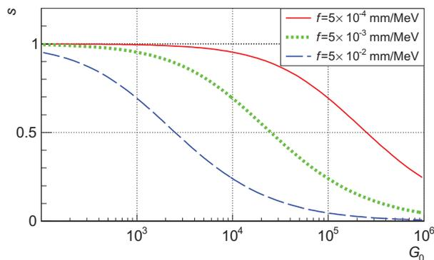
**Fig. 1.** Gain reduction factor ( $s$ ) calculated by the gain reduction model in Eq. (6) as a function of the multiplication factor ( $G_0$ ). The function is shown with three values of  $f$ . Here,  $dE/dl$  is fixed at the typical value of 20 keV/mm.
