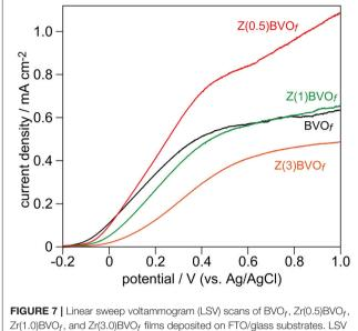
$Zr(1.0)BVO_f$ , and  $Zr(3.0)BVO_f$  films deposited on FTO/glass substrates. LSV curves were obtained in pH 6.86 phosphate buffer solution under photoirradiation of these thin films with a 300 W Xe lamp.
