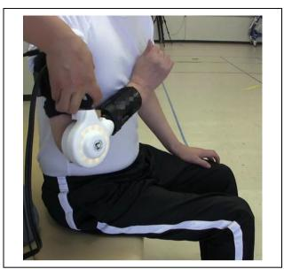
**Figure 5.** Elbow flexion exercises using the upper limb HAL-SJ in case 2. HAL-SJ: single-joint Hybrid Assistive Limb.
