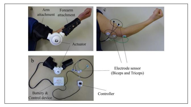
**Figure I.** (a and b) The upper limb HAL-SJ. HAL-SJ consists of the actuator in the elbow joint on the lateral side, arm/forearm attachments, battery and control device, controller, and electrode sensor. (c) Surface electrode sensors on the biceps and triceps. HAL-SJ: single-joint Hybrid Assistive Limb.
