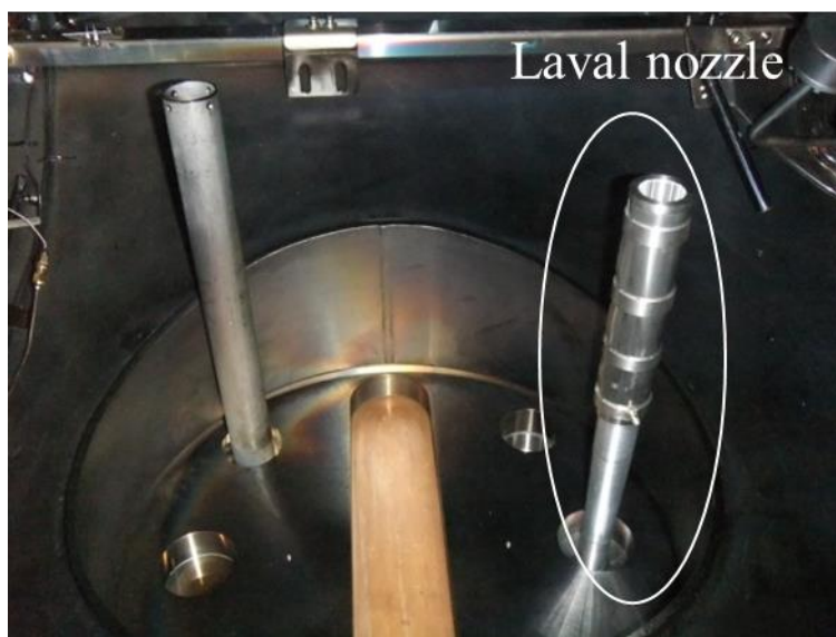
Fig. 2.4 SMBI system installed at the bottom of central-cell mid-plane.
