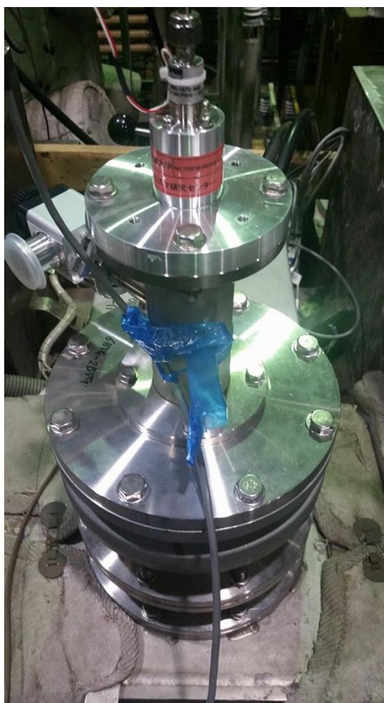
Fig. 2.5 (a) Photograph of the Laval nozzle, (b) New type SMBI system installed at the top of east anchor inner transition region.
