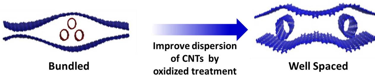
Fig. 14 Schematic of improved dispersion of CNTs in CNT/graphene composites.
