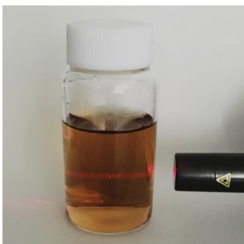
Fig.3 Photograph of aqueous suspension of oxidized MWNTs. The Tyndall effect is observed, indicating that the suspension is a uniform colloid.
