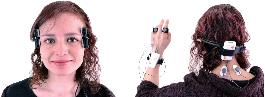
Figure 5.4: Wearables experiment 2 . From left to right, the EMG wearable, the usage of the Shimmer3 GSR on the hand, and the Shimmer3 GSR integrated on the EMG wearable to measure skin conductance from the neck.
