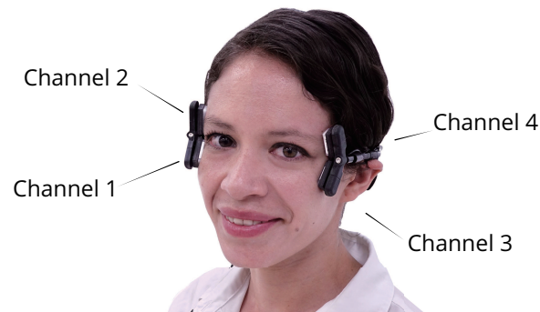
Figure 5.2: Wearable EMG channel position. The EMG wearable consists of four channels located as depicted in this figure. EMG activity on channels 1 and 2 was significantly different between the spontaneous and the posed blocks.
