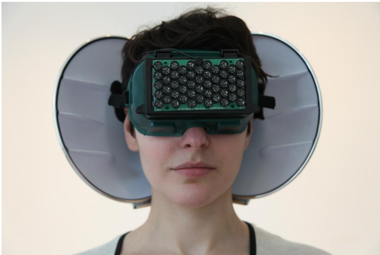
Figure 3: First Iteration of the Echolocation Headphones with Augmented False Auricles.
