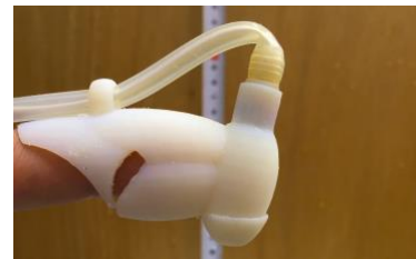
Figure 17: Cricket, vertical motor impeller fingertip actuator housing.
