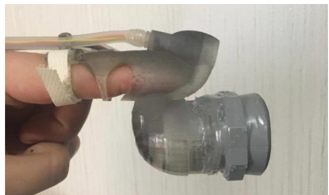
Figure 25: IrukaTact Sonar Tip
