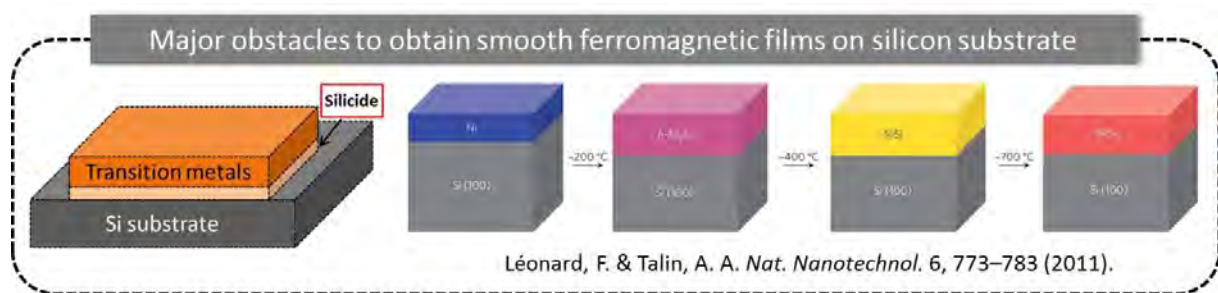
Fig. 5-2 Silicide formation problem in Ni-Si system.
