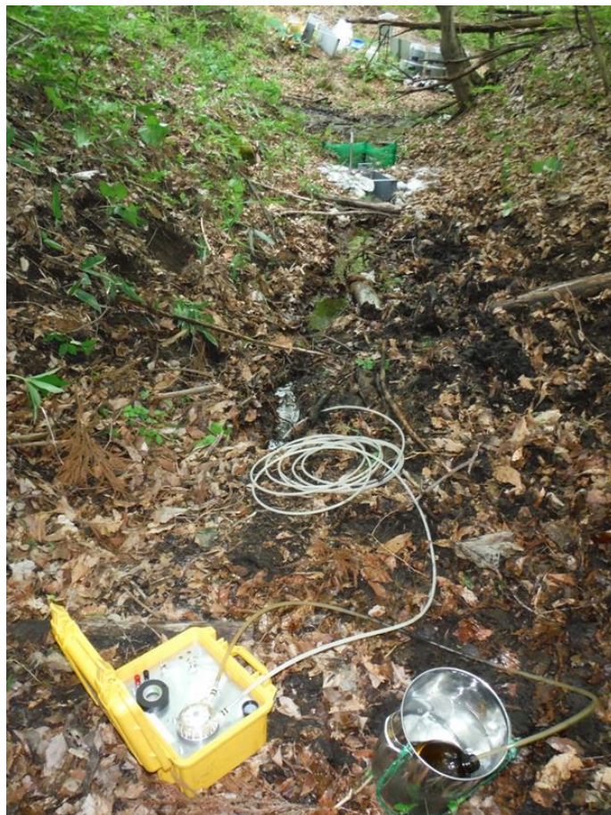
Figure 21. Picture of spring water sampling for SF 6 analysis with an appropriate pump that can prevent air contamination of sampled water.
