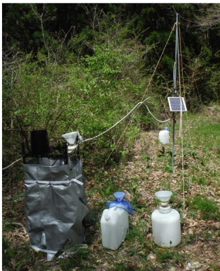
Figure 19. Installed rainfall monitoring system and rainfall collectors (RF in Figure 8).
