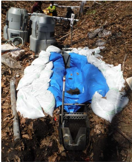
Figure 17. Installed V-notch weir and water table recorder for monitoring water discharge (P in Figure 8).
