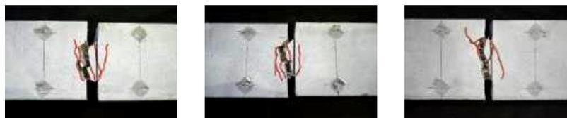
Figure 13. Crack patterns in specimens of notch set on two sides.
