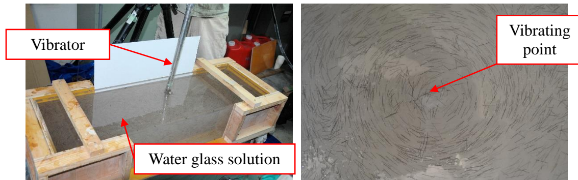
Figure 1. Example of fiber orientation after vibrating
