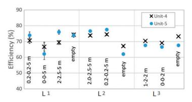
**Fig. 7.** Efficiencies of Unit-4 and Unit-5 plotted in chronological order. Horizontal is the layout number where the iron block thicknesses were changed. The three numbers attached to each data point are iron thicknesses placed between Unit-2 and Unit-4, Unit-4 and Unit-5, and Unit-5 and Unit-3. No iron was placed at "empty."
