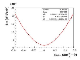
**Fig. 10.** Muon flux as a function of elevation angle  $\alpha$  measured using Unit-1 and Unit-2 only. No iron inserted. The curve is fitted with a simple function as described in the text.
