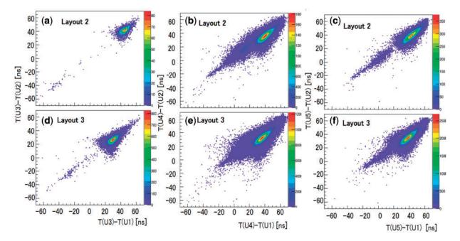
**Fig. 9.** Correlations of time differences between the third Unit (Unit-3, Unit-4, or Unit-5) with respect to Unit-1 (horizontal axis) and Unit-2 (vertical axis) in Layout-2 [a), b), c)] and in Layout-3 [d), e), f)]. The number of events is shown along the third axis.
