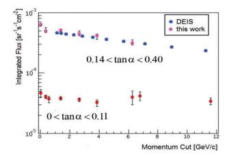
**Fig. 12.** Integrated muon flux as a function of the momentum threshold. The data of Ref. [2] are compared with this work in the range  $0.14 < \tan \alpha < 0.40$ . The data in the horizontal region  $0 < \tan \alpha < 0.11$  are also plotted.
