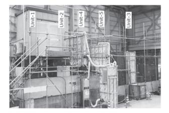
**Fig. 1.** Photograph of a detector setup (Layout-3 with one 2 m iron block inserted in front of Unit-3). Two 1 m  $\times$  1 m tracking units (Unit-1 and Unit-2) are located inside the storage hut at the top left, with another (Unit-3) behind the iron block at the right end (iron blocks not in use are placed further right). Two 1.6 m  $\times$  1.6 m units (Unit-4 and Unit-5) are in the middle, where piping for air-conditioning is seen.
