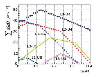
**Fig. 8.** The acceptance of the detector system as a function of the tangent of the track angle  $\alpha$ . The labels of the curves denote the three layouts (L1–L3) and the third unit used for tracking in addition to Unit-1 and Unit-2. Some other curves covering intermediate regions are not plotted.
