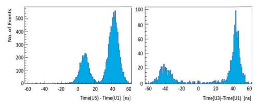
**Fig. 4.** Time differences (left) between Unit-5 and Unit-1, and (right) between Unit-3 and Unit-1. The front-arriving muons are distributed in the larger time-difference peak. Layout-1 configuration.
