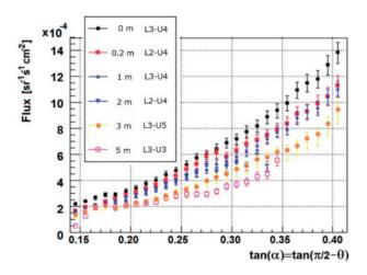
Fig. 11. Muon flux as a function of tan  $\alpha$  for different iron thicknesses used for comparison with the DEIS data. The iron thickness, layout number, and the third unit in the flux calculation are shown in the legend.
