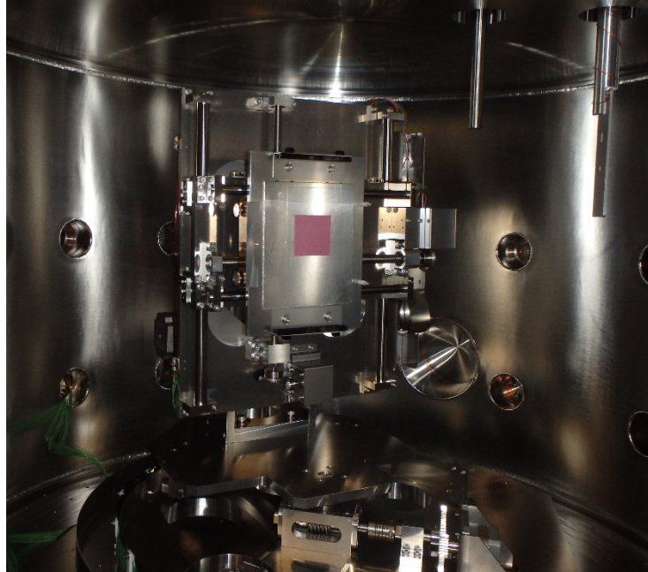
Fig. 2. Inside view of the main chamber, showing the target stage and the goniometer system.
