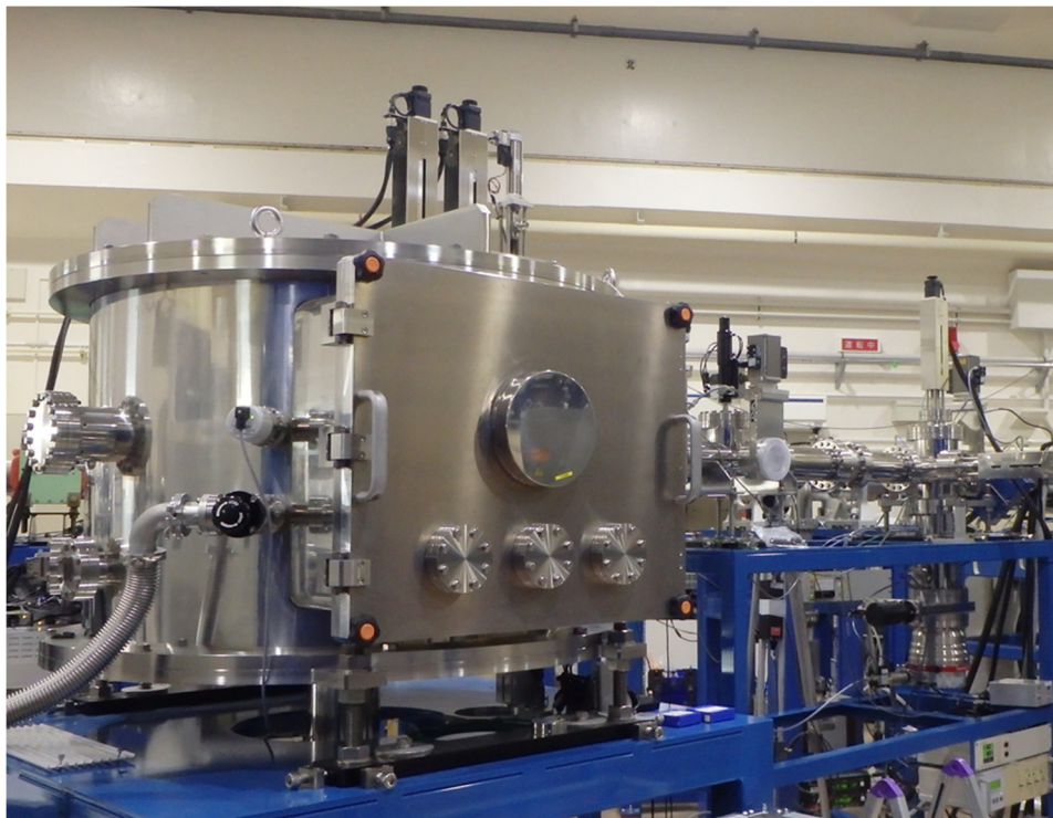
Fig. 1. Overall view of the irradiation-test chamber for semiconductor devices.
