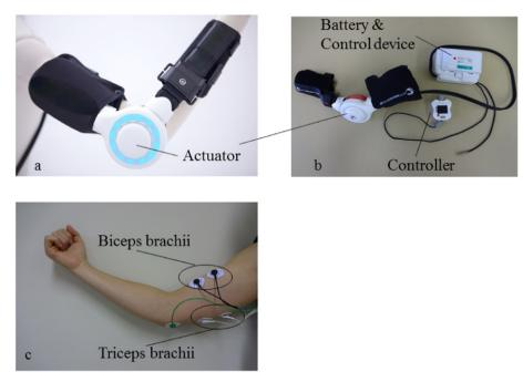
Fig. 1. a, b: Upper limb single-joint HAL (upper limb HAL-SJ). The upper limb HAL-SJ has the actuator (power unit) in the elbow joint on the lateral side. c: Surface electrodes on the biceps brachii and triceps brachii.
