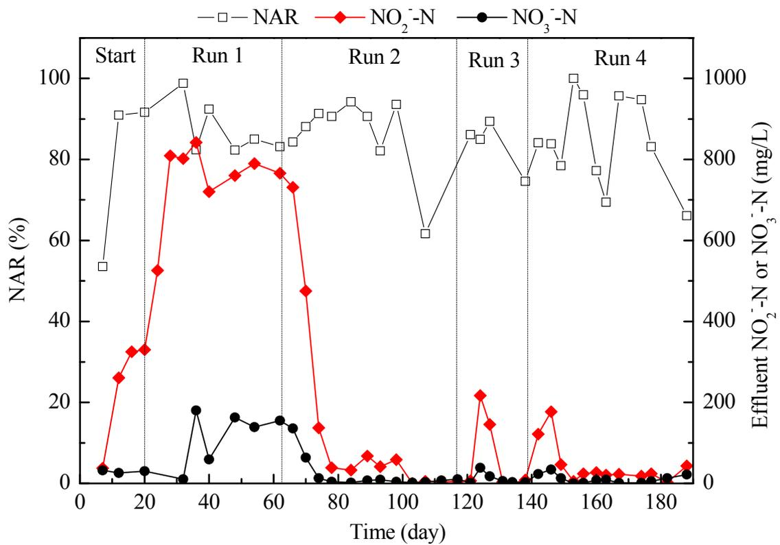
Figure 2-3. Changes of  $\text{NO}_2^-$ -N,  $\text{NO}_3^-$ -N and NAR in intermittently aerated sequencing batch reactor (IASBR) during Run 1 to Run 4.
