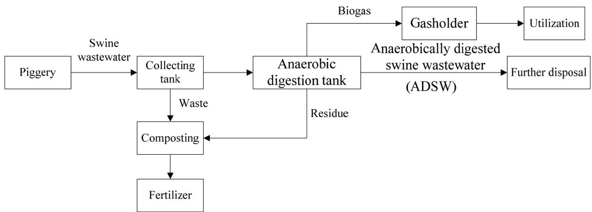
Figure 1-1. Typical treatment processes for swine wastewater in large-scale swine farms.
