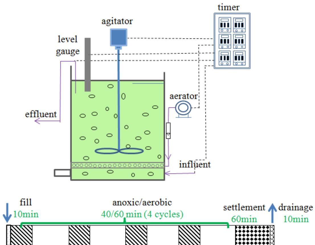
Figure 2-1. Schematic of lab-scale intermittently aerated sequencing batch reactor (IASBR) and its operation cycle.
