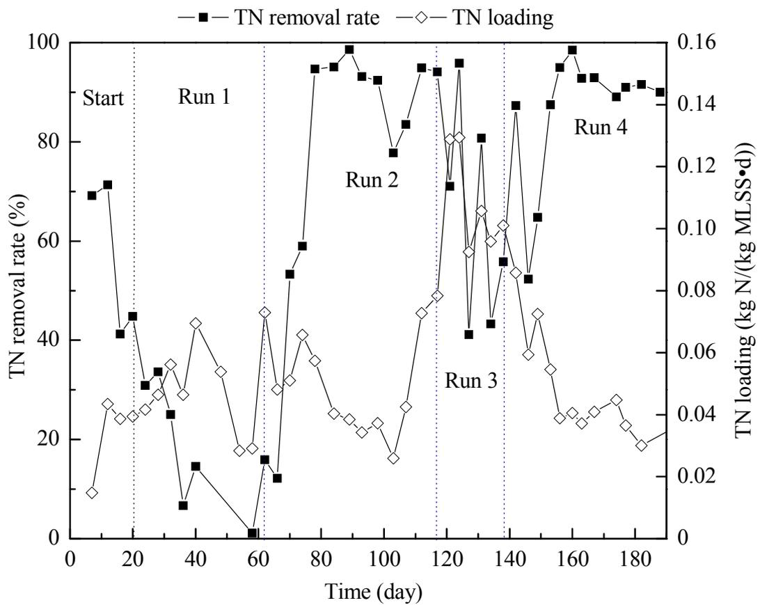
Figure 2-5. TN removal in intermittently aerated sequencing batch reactor (IASBR) during Run 1 to Run 4.
