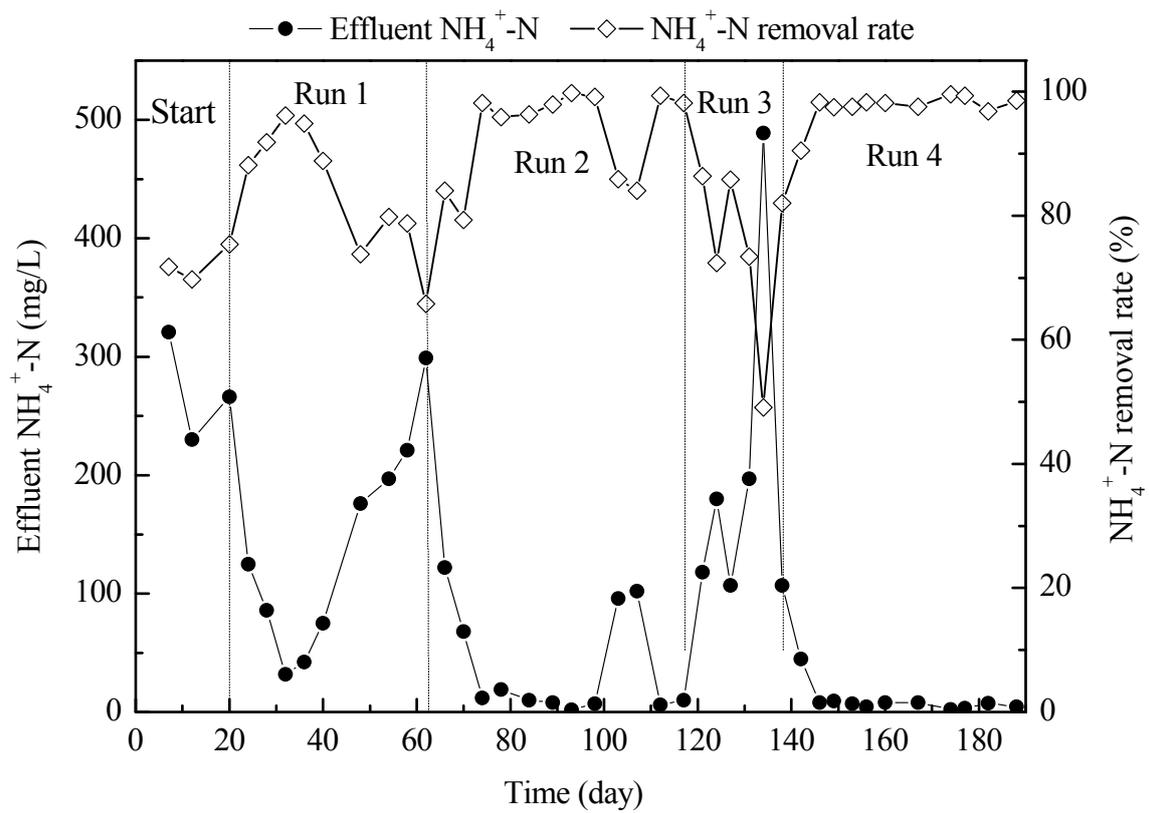
Figure 2-2.  $\text{NH}_4^+\text{-N}$  removal in intermittently aerated sequencing batch reactor (IASBR) during Run 1 to Run 4.
