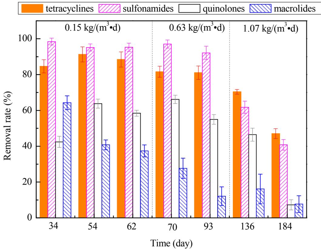
Figure 3-2. Variations in removal rates of antibiotics under different influent COD volumetric loadings.
