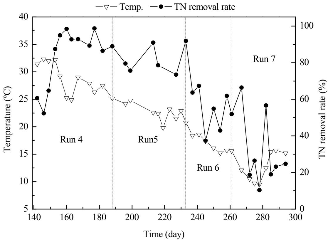
Figure 2-6. Effect of temperature on TN removal in intermittently aerated sequencing batch reactor (IASBR) during Run 4 to Run 7.
