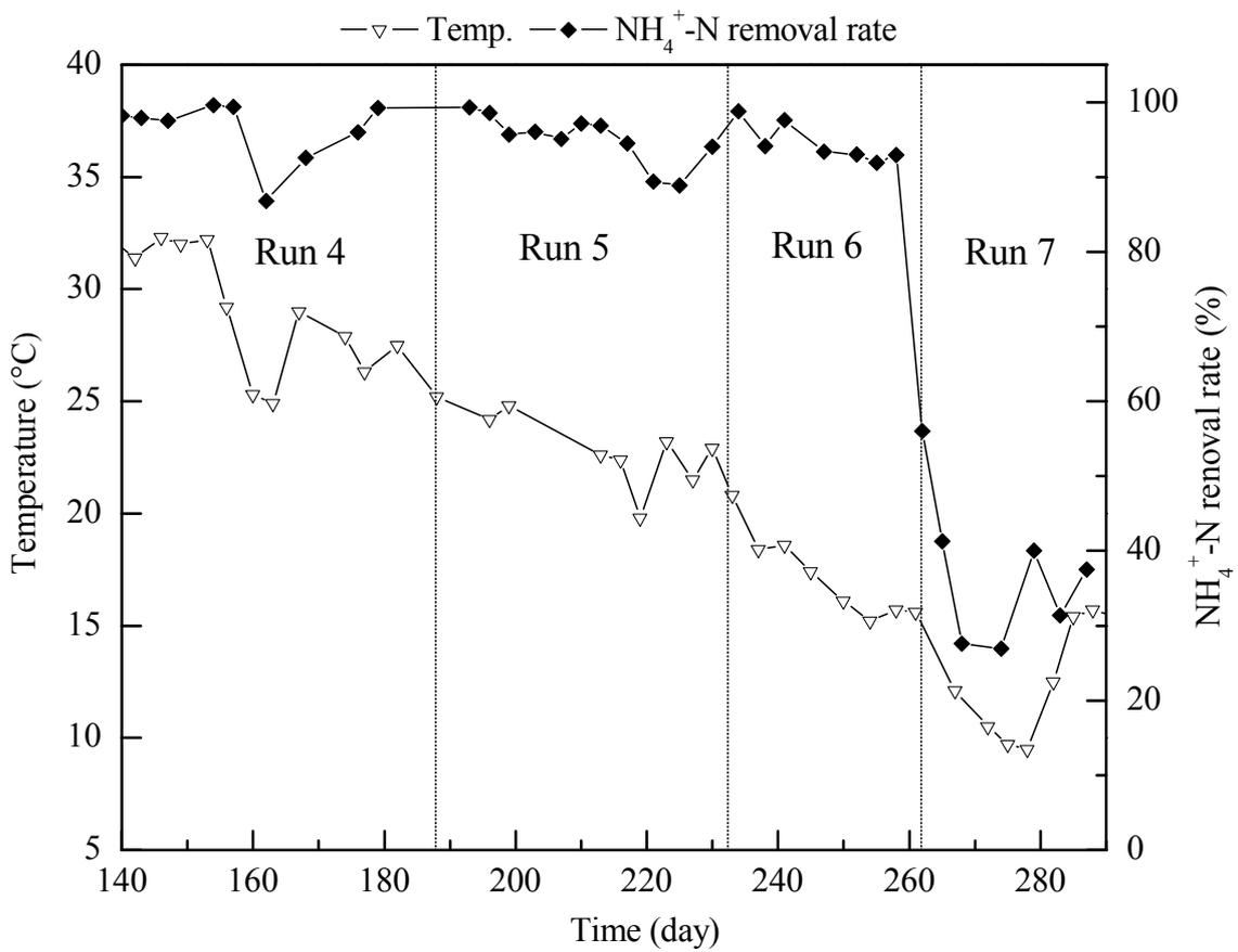
Figure 2-4. Effect of temperature on NH<sub>4</sub><sup>+</sup>-N removal in intermittently aerated sequencing batch reactor (IASBR) during Run 4 to Run 7.
