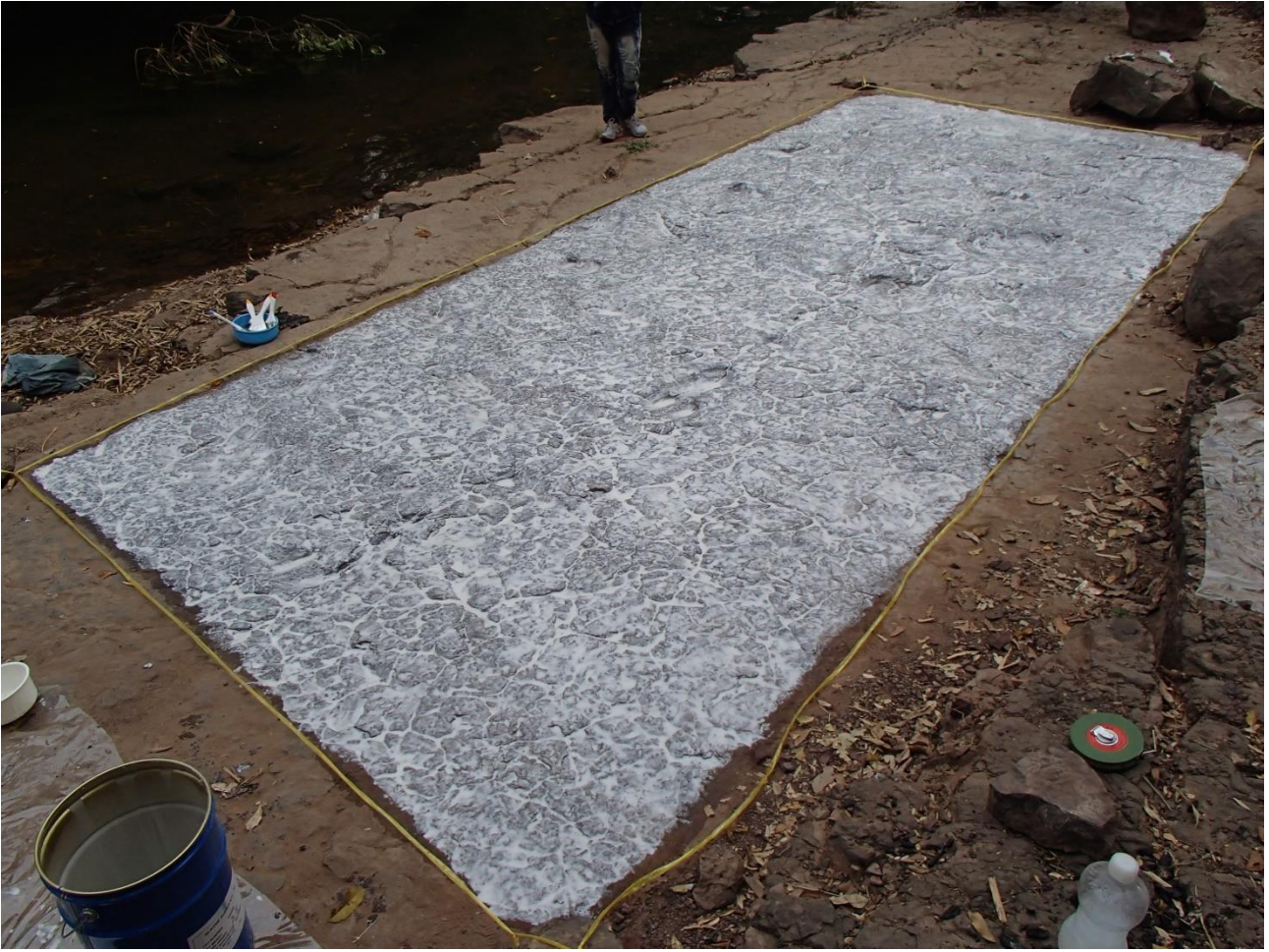
Figure 4 Photograph of making silicon replica (process 3).
