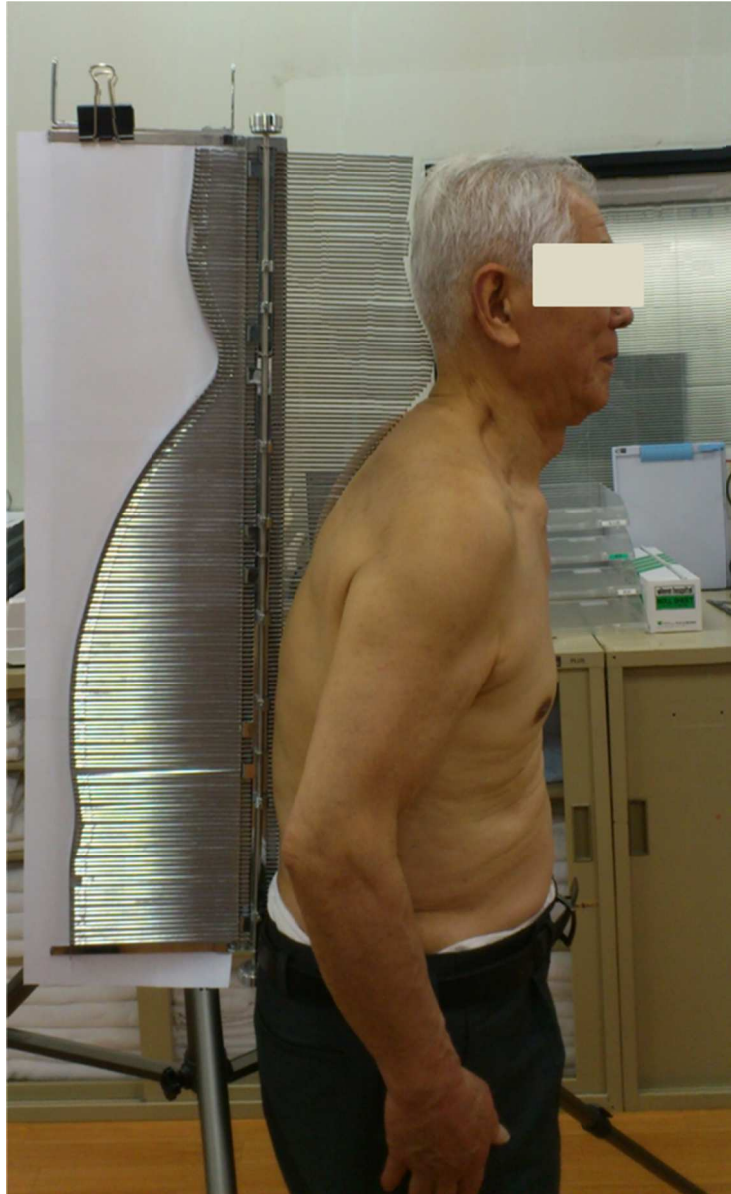
Figure 6.1 Measurement of spinal alignment by the conformateur type equipment.
