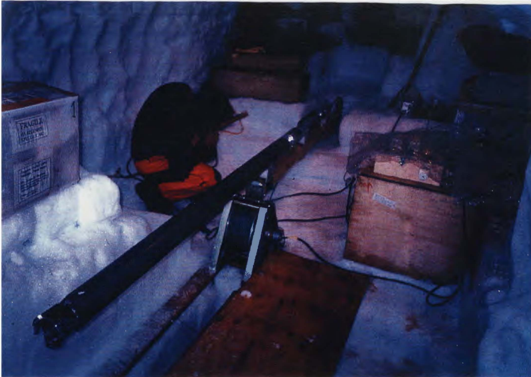
Figure 6. Tilted position of "Dokodemo drill No.1".
