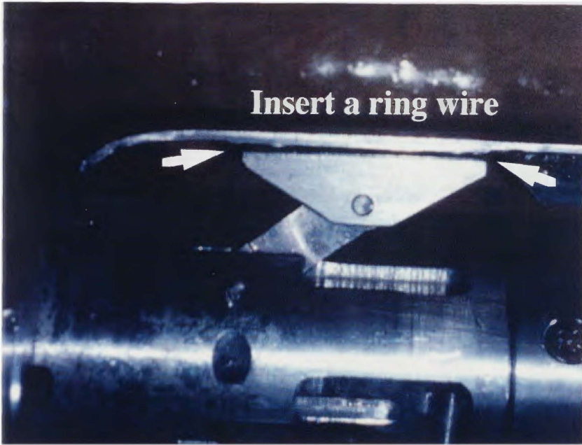
Figure 13. Expansion of blade by inserting a ring wire.
