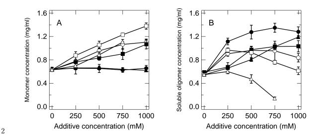
Fig. 5. Concentration of monomer (A) and soluble oligomer (B) of IgG after the heat treatment at 75°C for 2 min. The solutions contained 2.0 mg/ml IgG, arginine (closed circles), glucose (open circles), xylitol (closed squares), trehalose (open squares), glycerol (closed triangles), and sodium sulfate (open triangles). The measurements were performed three times, and the error bars depict the standard deviation of the mean.
