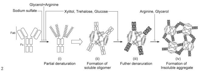
3 Fig. 7. Schematic illustration of the aggregation of IgG and the effect of additives.
