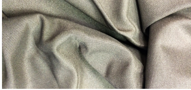
FIGURE 4.7: Conductive stretch fabric from Statex.
