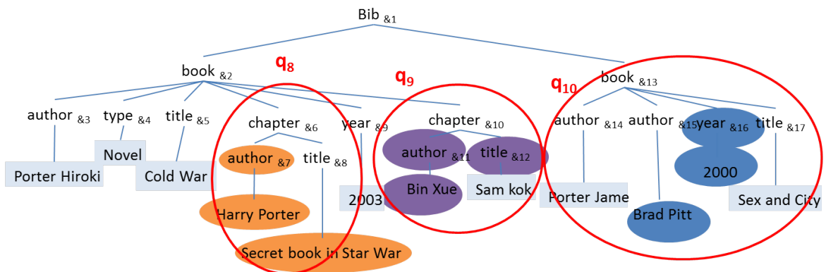
Figure 2.3: Querying keyword search q_8, q_9, q_{10} in XML data shown in Figure 2.2
