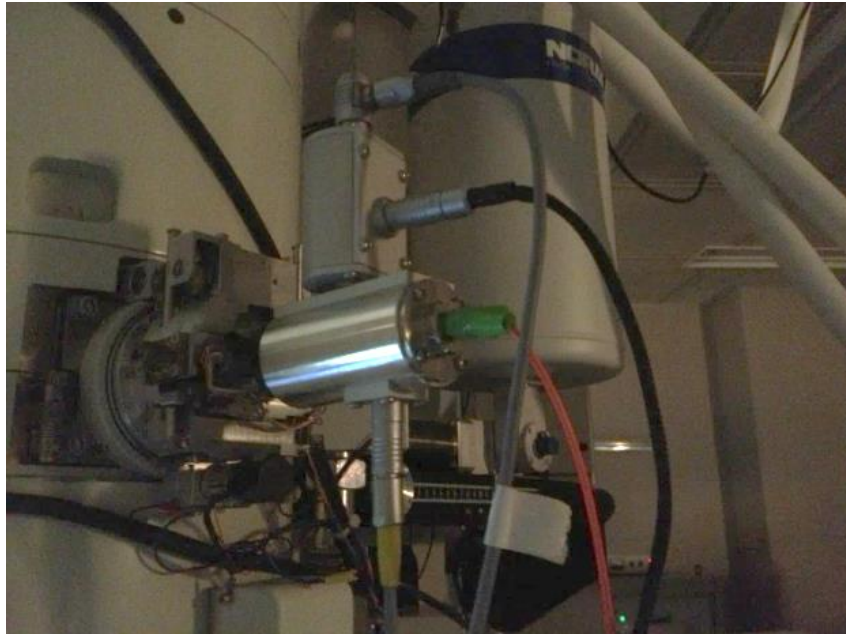
Figure 2.4: The holder has several I/O ports for in situ mechanical, electrical and optical access.
