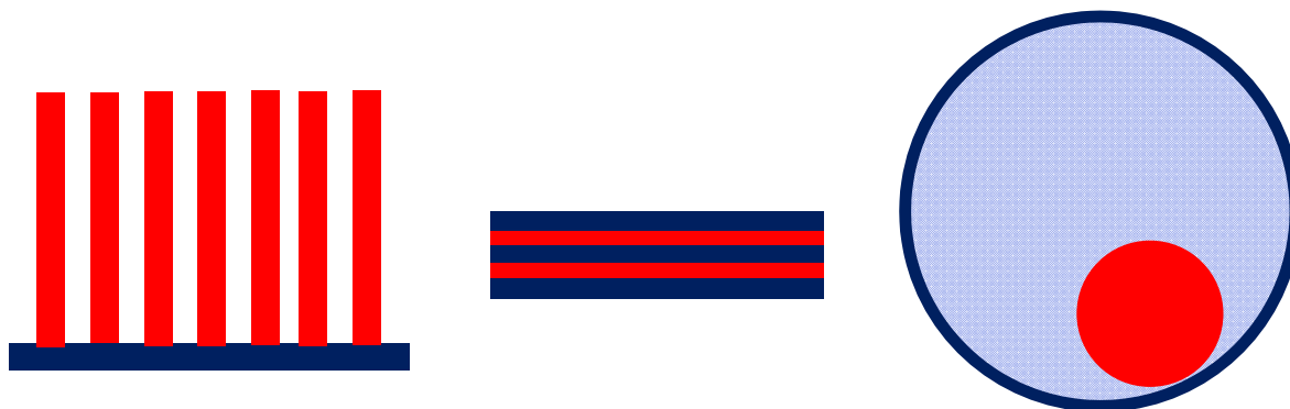
Figure 1.8: Designs for large volume expansion anode materials in batteries. Red color corresponds to the material with large volume expansion/shrinking during cycling, while material in blue color is the confinement material with low volume expansion rate and high mechanical strength.
