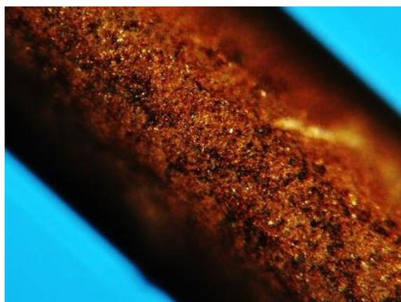
**Fig. 2-3** A pulverized sample set into the Lindemann glass capillary tube taken by an optical microscope.
