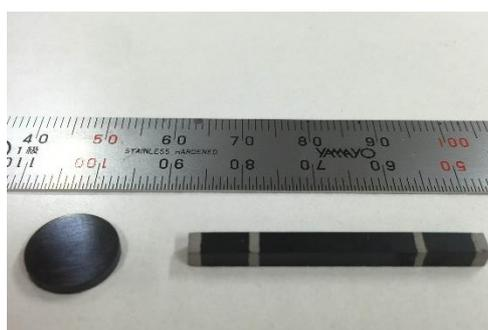
**Fig. 5-1** Sintered cylindrical pellet and rectangular specimen for measurements of electrical properties.
