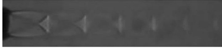
Figure 3.2 Wave patterns in a sonic under-expanded free-jet issuing from a tube run at nozzle pressure ratio P_0/P_b = 2.73 (ref. [11]). The barrel shock is clearly visible, as is the terminal shock wave (Mach shock wave). A skimmer can be used to transmit the central portion of the expansion into a second chamber (collimator chamber).
