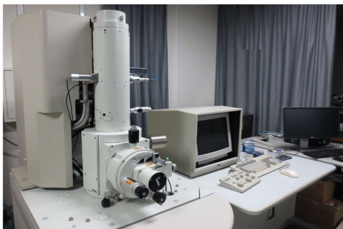
Figure 3-5. Scanning Electron Microscope FE-SEM (JSM-6330F, JEOL, Tokyo, Japan)
