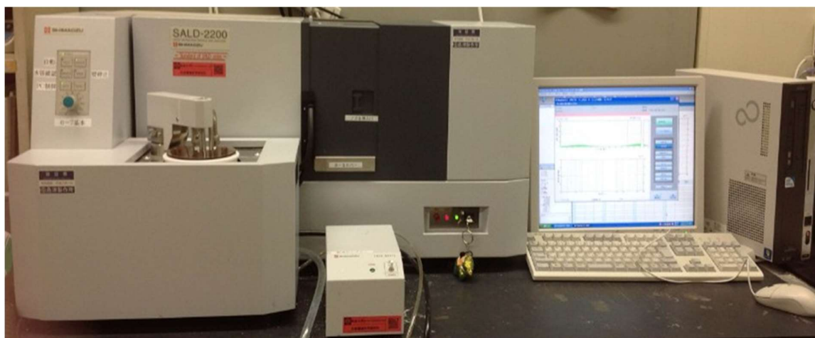
Figure 3-4. Laser diffraction particle size analyzer (SALD-2200, Shimadzu Corporation, Japan)
