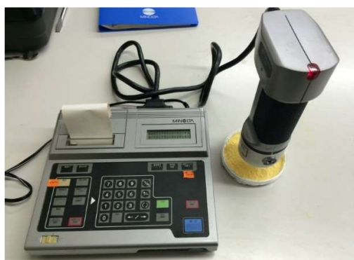
Figure 3-6. Colorimeter (CR-200, Minolta Co., Japan)
