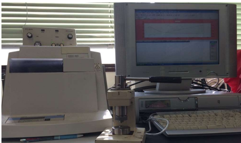
Figure 3-3. Differential scanning calorimetry (DSC) (DSC-60, Shimadzu, Japan)
