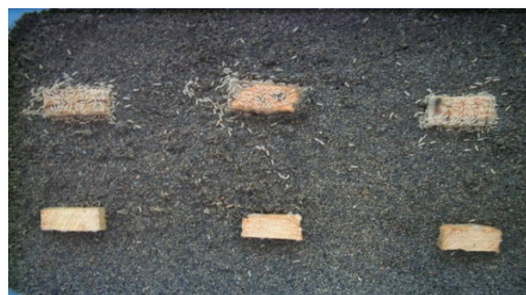
Figure 2. Termite aggregations on sound (upper three blocks) and decayed (lower three blocks) specimens of the same wood stake after the first 3 days of the choice feeding test. This aggregation pattern persisted until the end of the 14-day exposure period.
