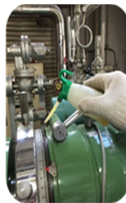
(2) Upper bearing and disk clearance adjustment
