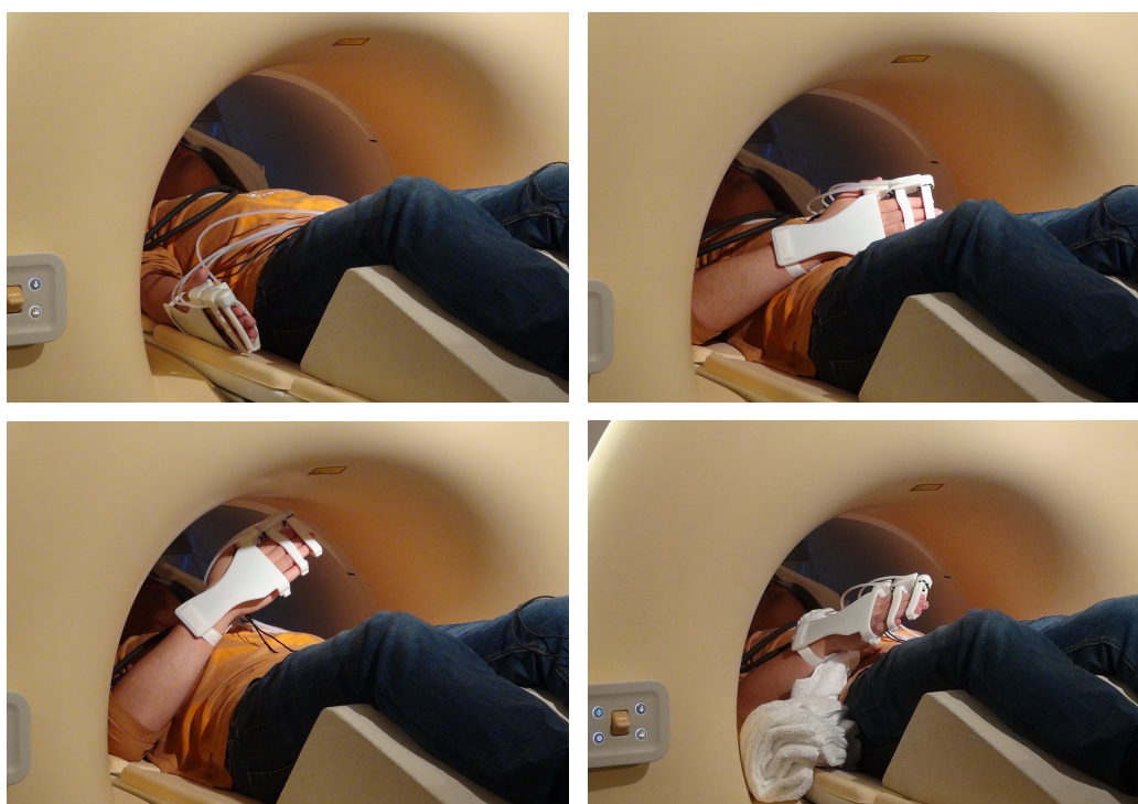
Figure 47 Hand unit that does not limit position and posture of participant's arm and hand.
