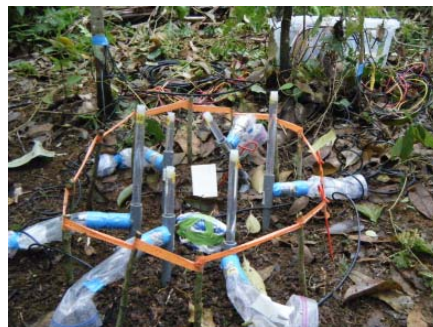
Fig. 2 Tensiometers for monitoring of rainwater infiltration and redistribution processes.
