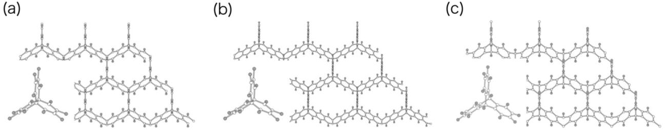
FIG. 1. Optimized structures of propellane networks with (a)  $C_6$   $sp^2$  and (b)  $C_{10}$   $sp^2$  C atoms, and (c) an iptycene network with  $C_6$   $sp^2$  C atoms. White and gray balls represent C and H atoms, respectively.
