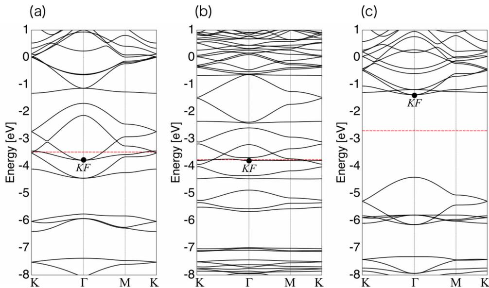
FIG. 2. Electronic structures of the hydrocarbon networks consisting of (a)  $C_6$  propellane vertices, (b)  $C_{10}$  propellane vertices, and (c)  $C_6$  iptycene vertices. The red dotted lines indicate Fermi levels. “KF” denotes the kagome flatband state.
