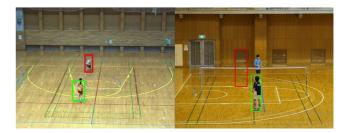
Fig. 2 TLD mis-tracking: tracking result without a net on a court (left) and with a net (right)
