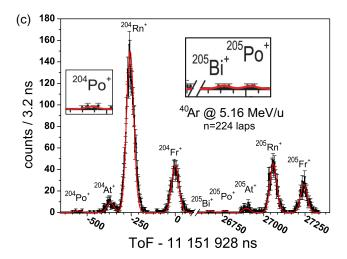
FIG. 2. Time-of-flight spectra observed using  $^{169}\mathrm{Tm}(^{40}\mathrm{Ar},~X)$  reaction at (a) 4.825 MeV/nucleon and (b, c) 5.16 MeV/nucleon. Ions made (a) n=148 laps, (b) n=223 laps, and (c) n=224 laps in the MRTOF-MS. The (a) A/q=205 and A/q=206 and the (b, c) A/q=204 and A/q=205 spectral peaks were observed simultaneously in single spectra. See text for details.
