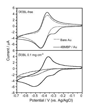
Fig. 4 Cyclic voltammograms of 4BMBP/Au (solid line) and bare Au (dotted line) in 1.0 mmol dm<sup>-3</sup> FMN solution containing no BL (a), and 0.1 mg cm<sup>-3</sup> BL (b). A 50 mmol dm<sup>-3</sup> phosphate buffer and 100 mmol dm<sup>-3</sup> KCl were added to the sample solution as a pH buffer and supporting electrolyte, respectively. The scan rate was 10 mV s<sup>-1</sup>.
