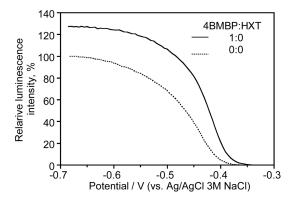
Fig. 5 Effect of the electrolysis potential on the relative luminescence intensity. Mixing ratios of 4BMBP and HXT were 1:0 (4BMBP/Au, solid line), 0:0 (bare Au, dotted line). The results of 1:1 (4BMBP-HXT/Au) and 0:1 (HXT/Au) are not shown (no luminescence).
