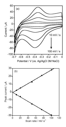
Fig. 3 (a) Cyclic voltammograms of the 4BMBP/Au mesh electrode in 50 mmol dm<sup>-3</sup> phosphate buffer and 100 mmol dm<sup>-3</sup> KCl solution at pH 7.0. The scan rates were 10, 20, 50, 75 and 100 mV s<sup>-1</sup>. (b) Scan rate dependence on the redox currents. The closed circles indicate the cathodic peak currents and the closed triangles indicate the anodic peak currents. The redox currents were obtained from Fig. 3(a). The solid lines indicate a first-order regression line.
