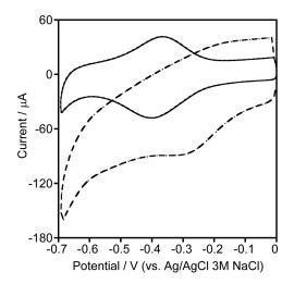
Fig. 2 Cyclic voltammogram of 4BMBP/Au-mesh in 50 mmol dm<sup>-3</sup> phosphate buffer and 100 mmol dm<sup>-3</sup> KCl solution. The solid line and dashed line indicate the result of the 4BMBP/Au and the bare Au, respectively. The pH value was adjusted to 7.0. The scan rate was 100 mV s<sup>-1</sup>. The Au mesh electrode was used in this experiment.
