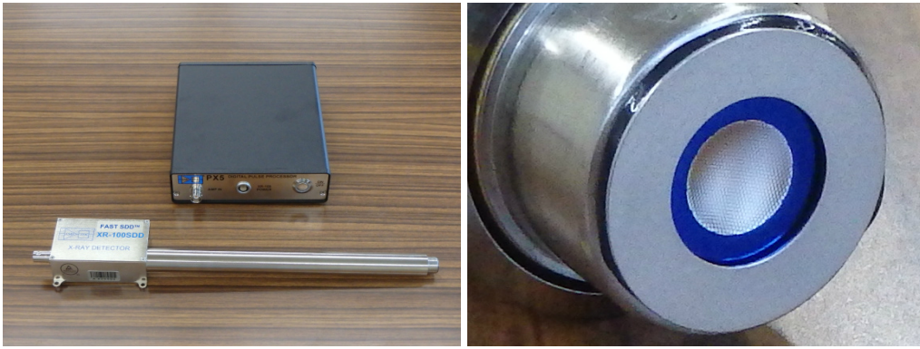
Fig. 1. Photographs of the silicon drift detector XR-100FastSDD with digital pulse processor (Amptek Inc., US) (left). An entrance window is made of silicon nitride ( \text{Si}_3\text{N}_4 ) with a thickness of 40 nm for observing characteristic X-rays from light elements (right).
