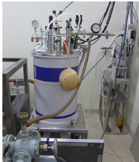
Fig.1. Setup of the measurement system with superconducting magnet.
