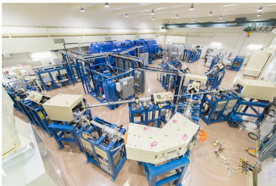
Fig. 4. Photograph of the 6 MV Pelletron tandem accelerator under construction in the accelerator room.
