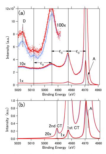
FIG. 5. Experimental (a) and simulated (b) Ti 1s spectra, shown at different vertical magnifications. In the highest magnification (100×) experimental spectra, the data points are shown by dots, and 30 point smoothed spectra are shown by solid curves. The gray and black (thin blue and red) represent the  $\beta$  and  $\lambda$  phases, respectively.
