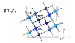
FIG. 3. Unit cells of  $\beta$  phase [(a) and (c)] and  $\lambda$  phase Ti<sub>3</sub>O<sub>5</sub>. The three different sites of Ti atoms are indicated as Ti(1), Ti(2), and Ti(3).
